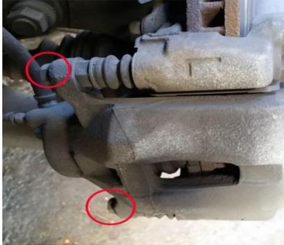
Figure 1. Brake caliper retaining bolts location
