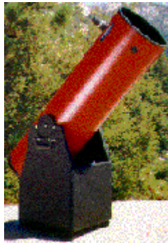
Figure 2. Dobsonian alt-azimuth mount [6].
