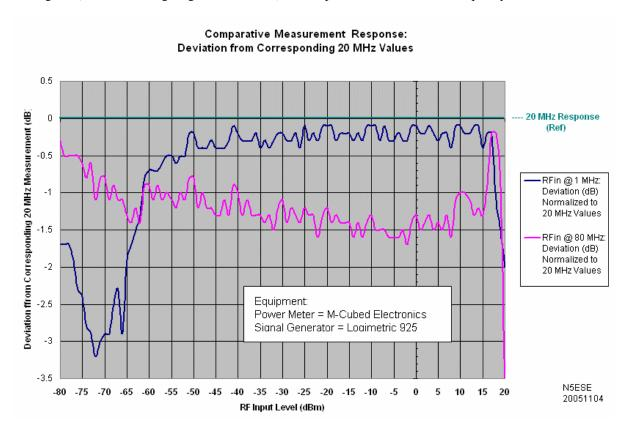
Note, when observing these results, that these curves could easily be shifted upward by the FPM-1's frequency correction algorithm, which was not in effect with these data. So, when looking at these curves, focus primarily on the changes from left to right.
