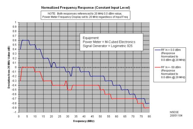
Based on the two curves above, it can be seen that in the range from 1 through 80 MHz, all measurements were within 1 dB, with the raw response generally decreasing with rising frequency, which is to be expected. It should be nearly level at 0 dBm in the released version of the FPM-1, if one uses frequency correction by telling the power meter what frequency is being applied.
