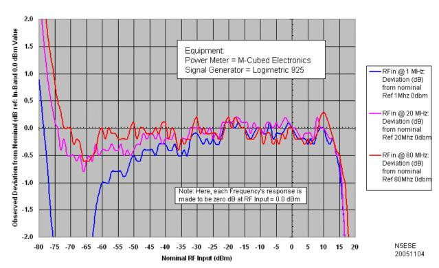
From the chart at 20 Mhz (where the 0.0 dB calibration was done), the dynamic measurement range is seen to be:
