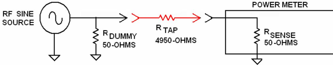
**SIMULATION: IDEAL 40 dB TAP ATTENUATOR & IDEAL POWER METER INPUT**
