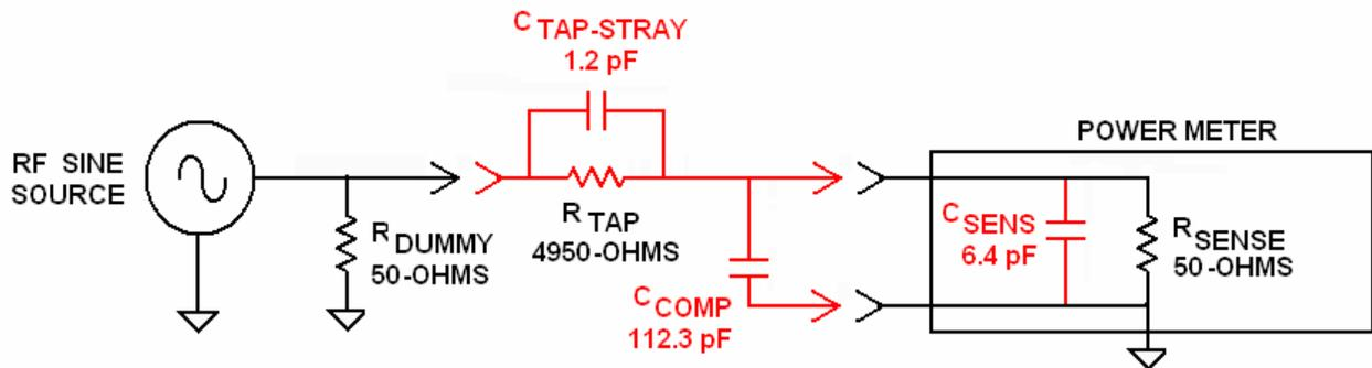
**SIMULATION: IDEAL 40 dB TAP ATTENUATOR & STRAY CAPACITANCE IN SENSOR**
