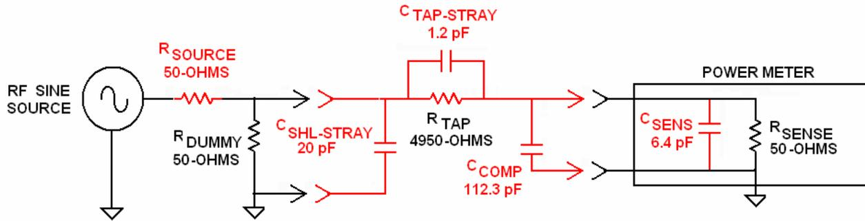
**SIMULATION: FULLY COMPENSATED 40 DB TAP ATTENUATOR WITH KEY STRAY CAPACITANCES**
