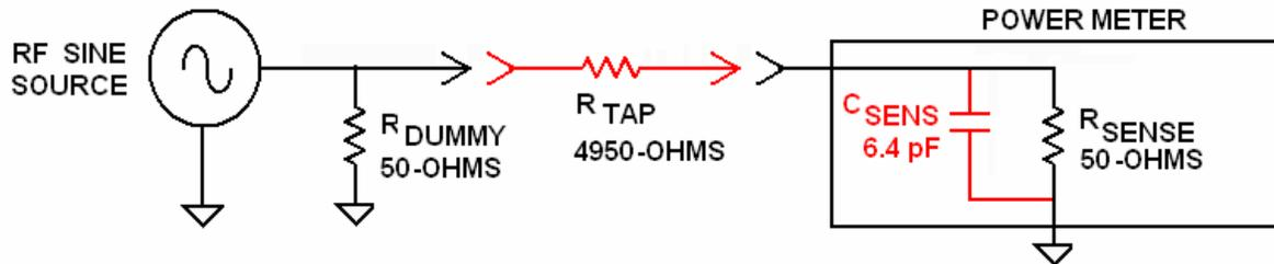
**SIMULATION: IDEAL 40 dB TAP ATTENUATOR & STRAY CAPACITANCE IN SENSOR**
