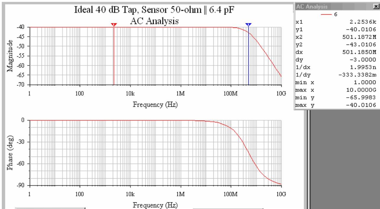
We have yet another stray capacitance we haven't considered yet, that of the tap itself. As can be seen in the schematic below,  $C_{TAP-STRAY}$  and  $C_{SENS}$  form a voltage divider of their own, but the division ratio is not 40 dB, and that leads to trouble.
