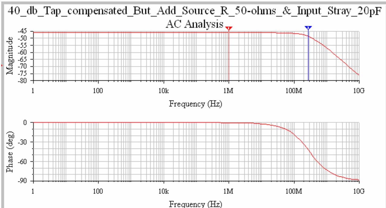
As you can see, the -3 dB point is just under 200 MHz, and the -1 dB is about 150 MHz. Also notice the graph now shows the attenuation as -46 dB. This is because there is 6 dB "loss" in the resistor  $R_{\text{SOURCE}}$ . It's not really a loss, it's just an artifact of source simulation.
